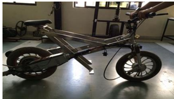
Figure 7: Proposed design of the e-bike (scissor frame)
