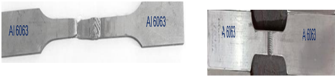
Fig 4.1.1 Tensile Test Specimens after testing on UTM of Al -6063 & Al-6063 Load vs Displacement
