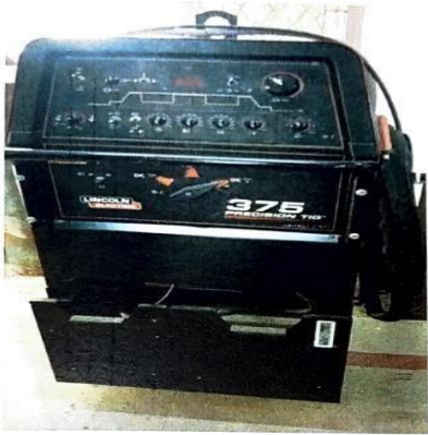
Fig 3.4 LINCOLN 375 welding machine
