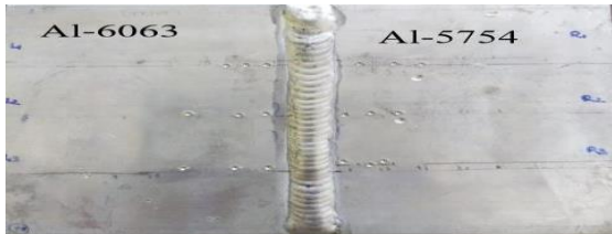
Fig 4.2.5 Rockwell Hardness Test on Weldment AL-6063 & Al-5754
