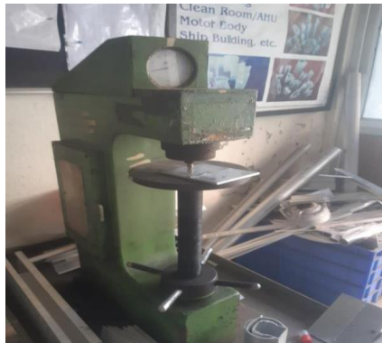
Fig 3.9 Rockwell Hardness Testing Machine
