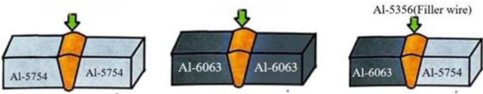
Fig 3.2 Weld Plates Preparation and Welding Procedure
