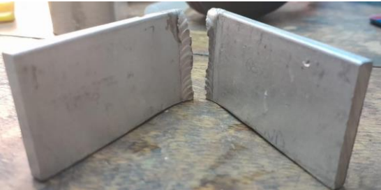
Fig 4.3.1 Bend Test of AL-6063 & Al-6063 (Sample 1)
