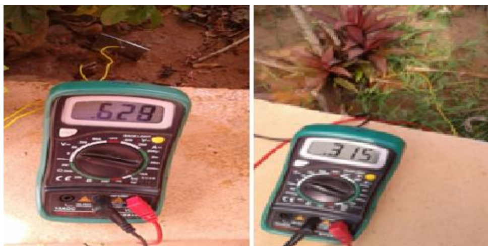
Figure 3. Different Electrodes in Chethy Plant with different electrodes (Zn-Fe and Fe-Al).
