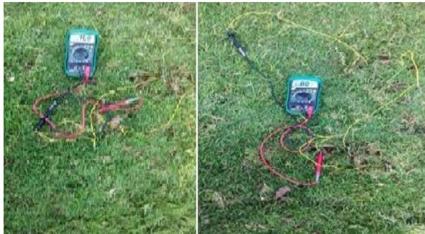
Figure 4. Electrode Zn-Fe into the roots of the grass
