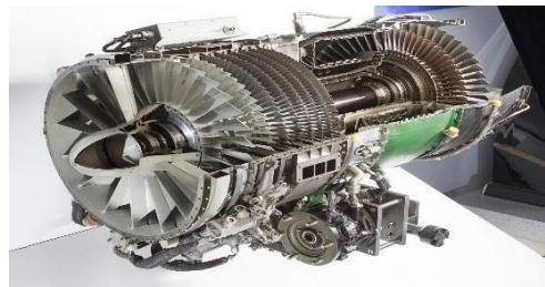
Figure 1.1: General Electric J85 Cutaway with Axial Flow Compressor [2]
