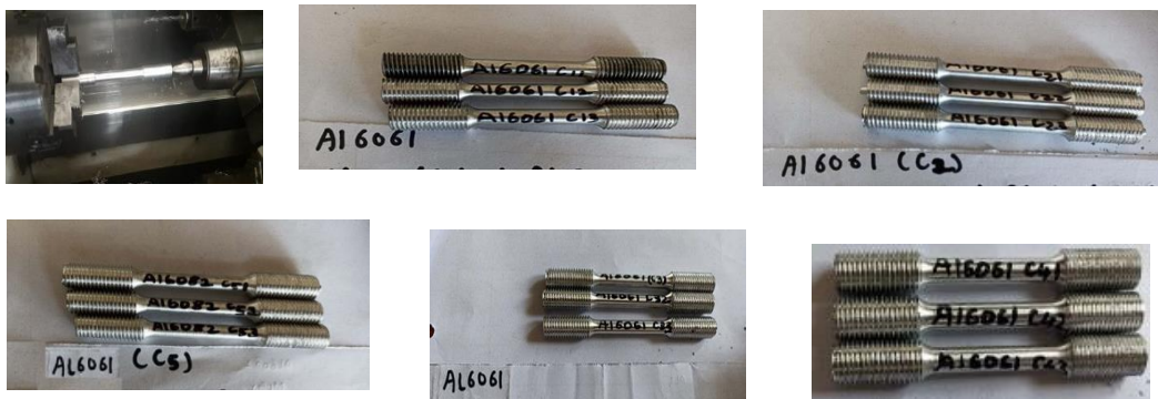
Figure 2. (a) Al6061-Al 2 O 3 /MoS 2 Metal matrix composites Tensile specimens machining with varying composition, (b) C1 Pure Al6061, (c) Al6061/5% Al 2 O 3 -5% MoS 2 , (d) Al6061/10% Al 2 O 3 -5% MoS 2 , (e) Al6061/15% Al 2 O 3 -5% MoS 2 , (f) Al6061/20% Al 2 O 3 -5% MoS 2
