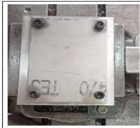
Figure 1: Fixture designed for mounting the work piece]
