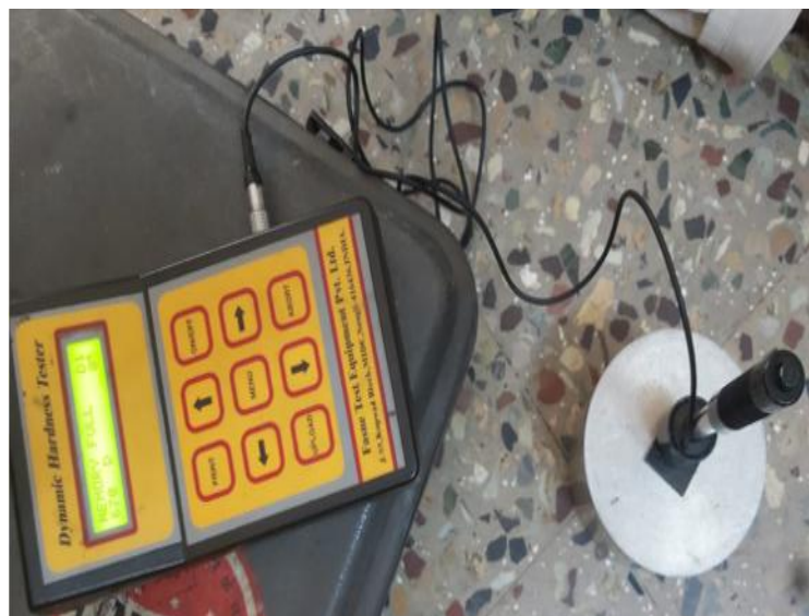
Figure. 7 Shore D Hardness Test
