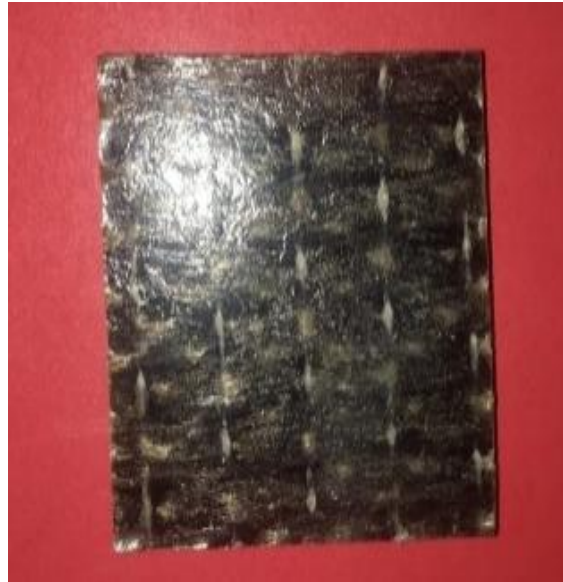
Figure. 6 Shore D Hardness Test Specimen
