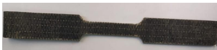
Figure. 2 Specimen Before Tensile Test
