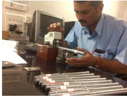
Figure 2. Surface Roughness Testing by Accurate Lab
