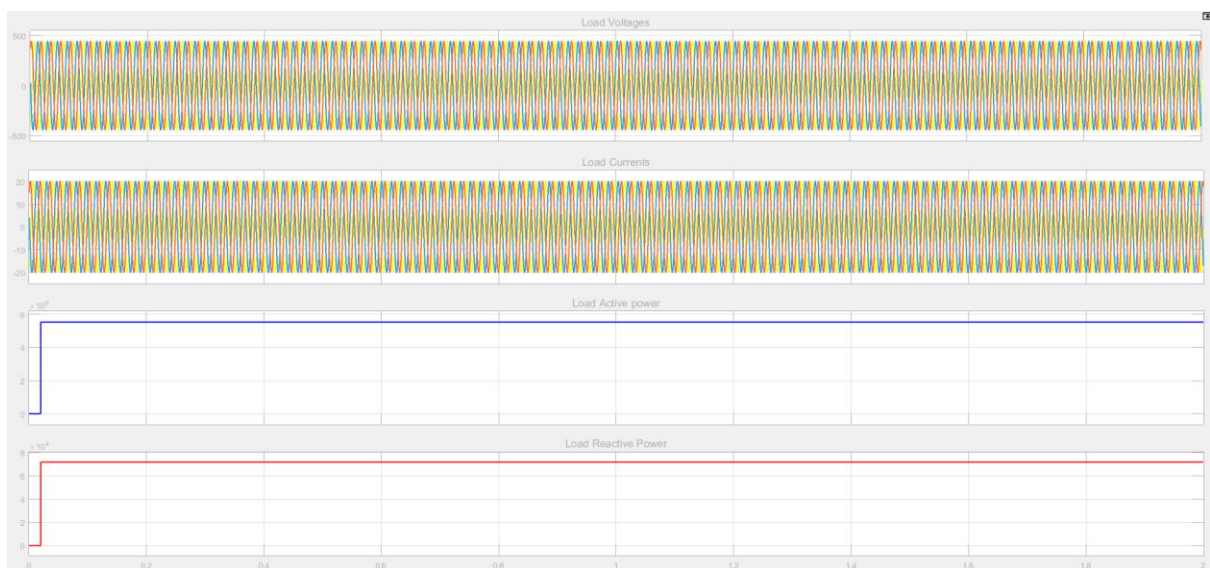
Fig10. Load Voltages, Currents and Active Reactive Power with fuzzy system
