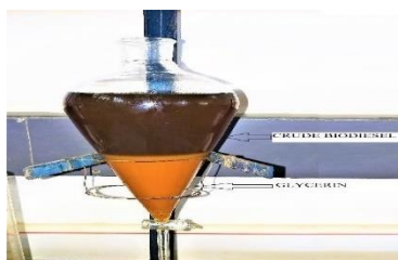
Fig.5: Crude biodiesel after transesterification process
