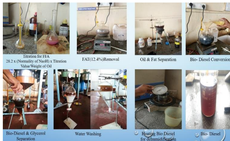
Fig 6: Biodiesel production process.
