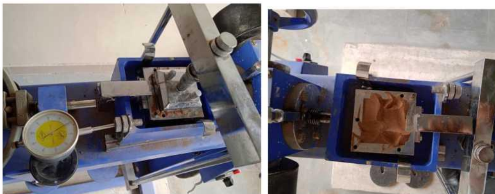
Figure 1: Direct shear test apparatus: (a) test setup; (b) shear box
