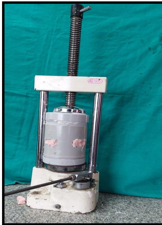
Fig 11 – Hydraulic press used to compress the flask and promote flash
