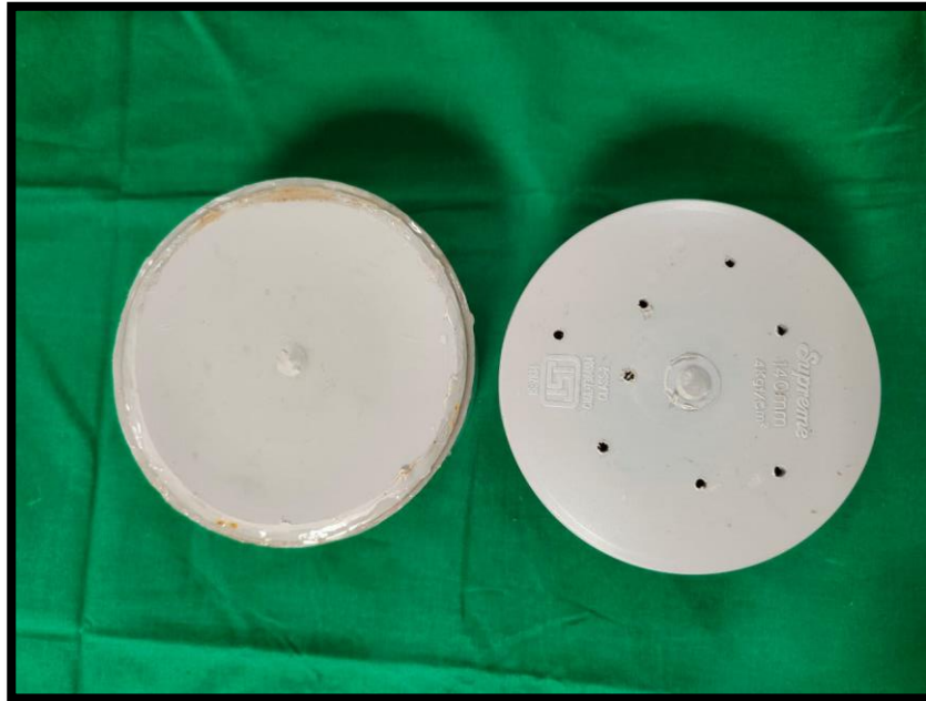
Fig 8 – Escape vents made on the lid
