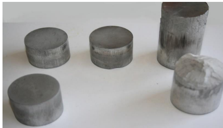
Figure 1: Samples from stage 1, where the parts on the left are sound and the parts on the right are broken or scratched due to not following the diameter to height ratio.
