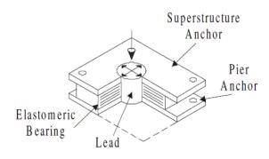
Figure 1. Lead-rubber bearings.
