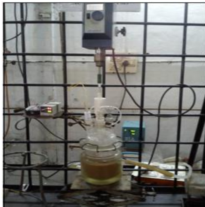
Fig.1. Four necked jacketed batch reactor for acid hydrolysis treatment
