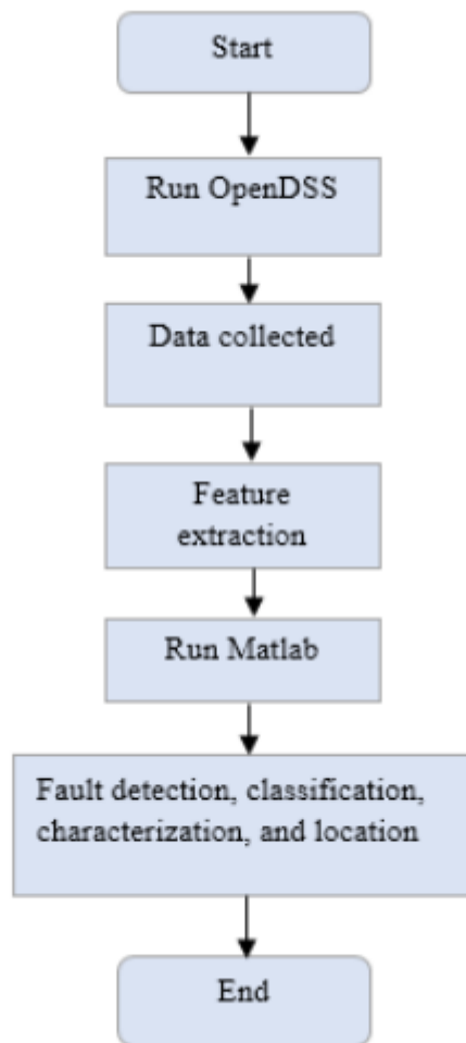
Fig 4: Fault detection, classification and location flowchart
