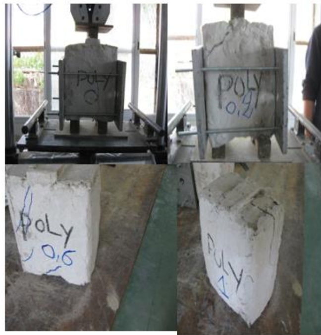
Fig.8: Final states of failure for triplet shear tests under different value of pre-compression for reinforced shear triplets (RST)
