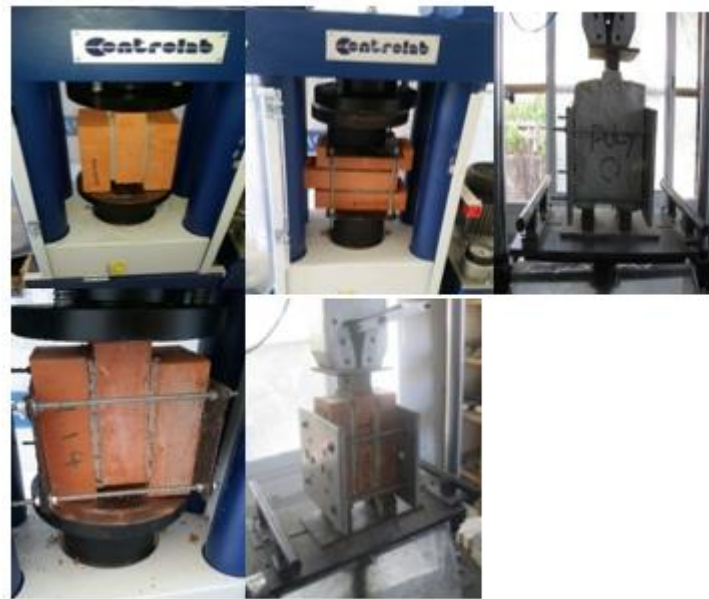
Fig.2: Test setup of shear triplet test
