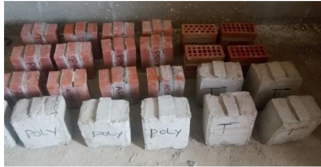
Fig. 4: Application of FRMC strengthening to shear
