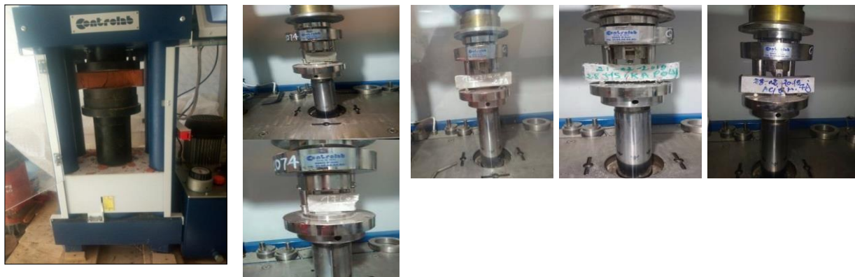
Fig.1. Three-point bending test and compressive test for mortar prisms and brick units
