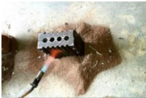
Fig 2: a) Pre Heating of Metal Mould b) Pouring of Molten Metal to Metal Mould
