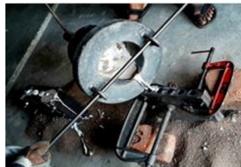
Fig 2: a) Pre Heating of Metal Mould b) Pouring of Molten Metal to Metal Mould
