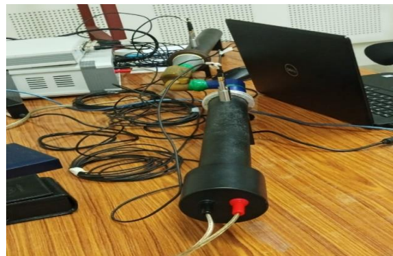
Fig 7: Impedance tube connected to DAQ equipped sensors
