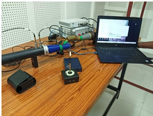
Fig 4: DAQ connected to PC and muffler
