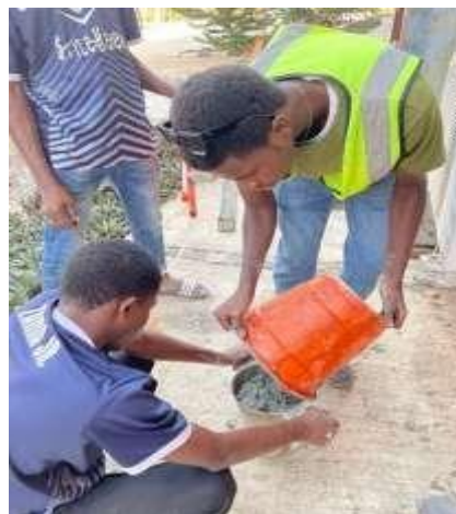
Figure 1. Slump flow test in progress
