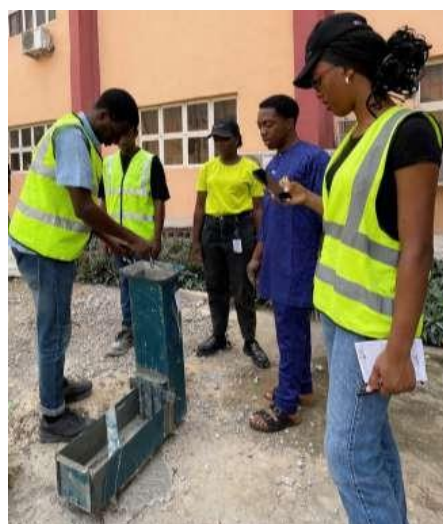
Figure 3. L-Box test in progress
