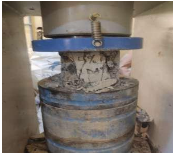
Figure 4. compressive strength test
