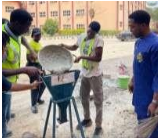
Figure 2. V-Funnel test in progress
