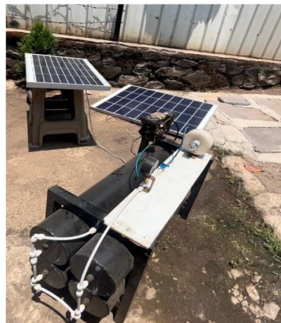
Prototype Model of Solar-Based Compressed Air for Energy Generation
