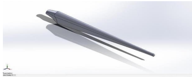
Figure 1: 3D CAD model of a HAWT blade designed with NACA 4412 airfoil.
