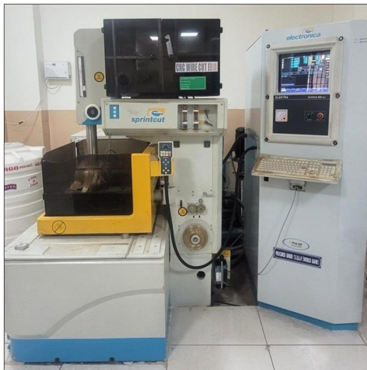
Figure 1. Electronica ELPULS 40A DLX Sprint-cut CNC WEDM machine
