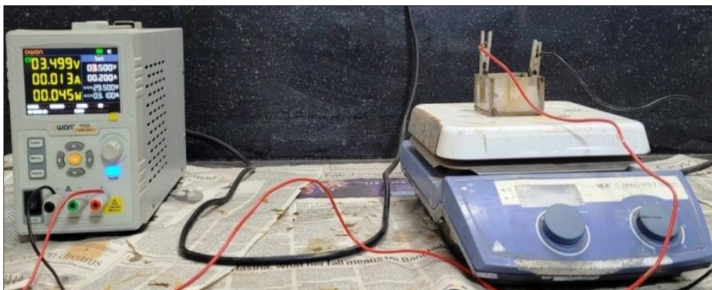
Figure 2. ECD set-up for HA coating
