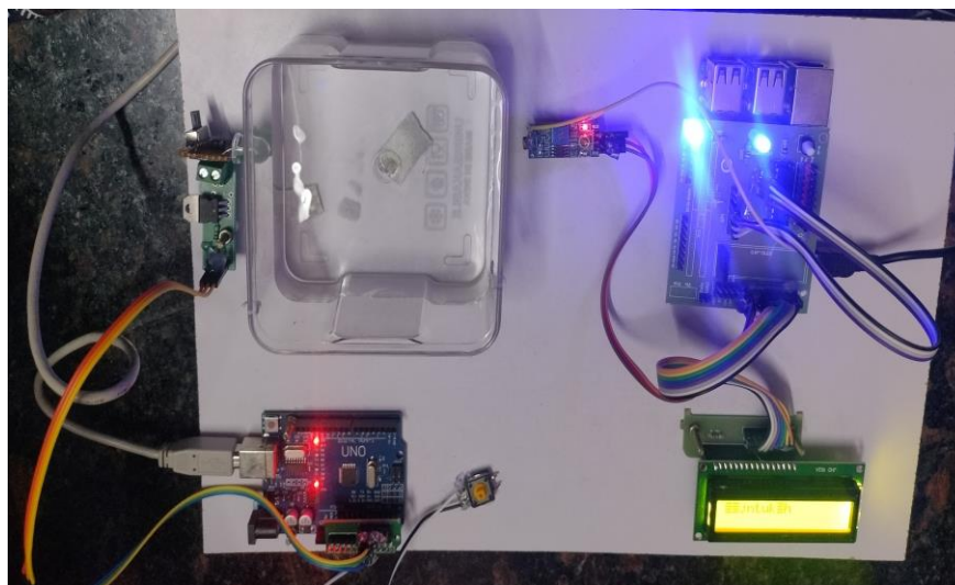
Fig. 6. First image of the underwater optical wireless communication prototype showing transmitter and receiver arrangement in the experimental water tank.
