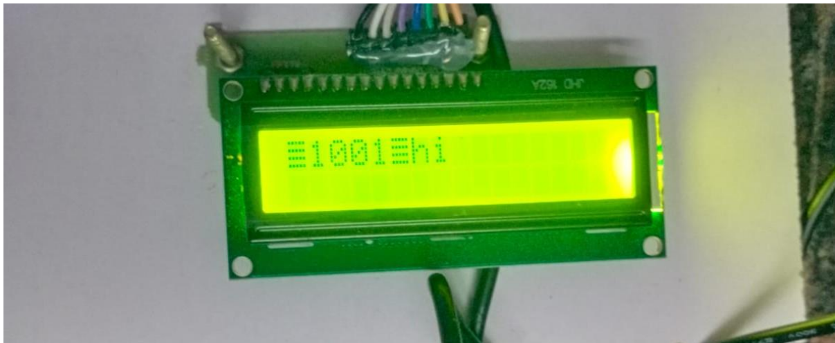
Fig. 9 Screenshot of received and decoded data shown on the LCD and monitor, evidencing successful underwater optical communication.
