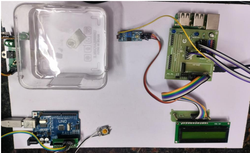
Fig. 7. Second image of the prototype emphasizing the interfacing of MCP3208 ADC with the Raspberry Pi for digital signal processing.
