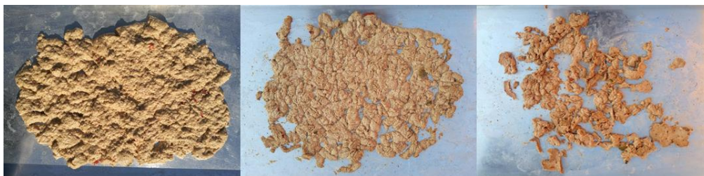
Fig. 3 Evolution of the aspect of synthetic sludge during drying (from the left picture at the beginning of the tests to the right picture at the end of drying)
